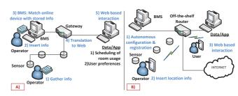
Figure 1. Commissioning process of sensors as currently carried out (A) and as envisioned utilising CoAP/IPv6 technology (B).
