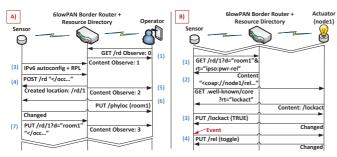
Figure 2. Detailed operation of the CoAP/IPv6 commissioning process (A) and the CoAP based distributed control application (B).
